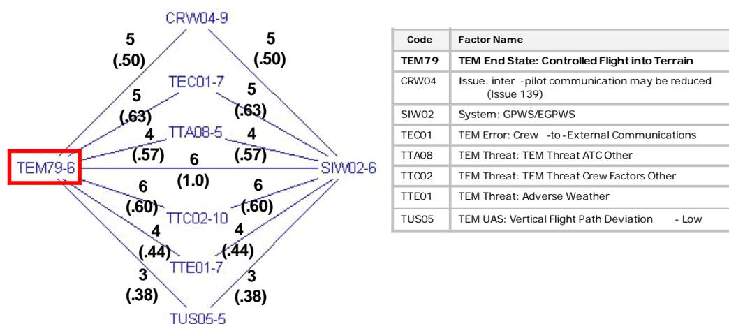
Figure 1. The co-occurrences identified in Controlled Flight Into Terrain accidents.
